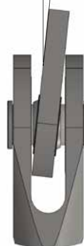
Additional misalignment with spherical bearing
